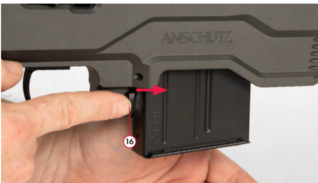
Fig. 30 Pushing the magazine release lever forward
