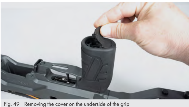
Fig. 49 Removing the cover on the underside of the grip
