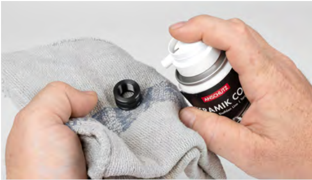
Fig. 58 Cleaning and lubricating the threaded bushing
